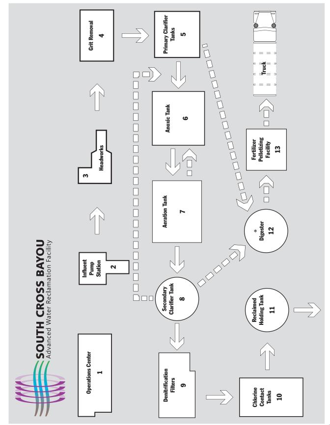
Dotted arrows represent the flow of solids/sludge whereas solid arrows represent liquids/water. \*For simplicity, not all processes are graphically represented.
