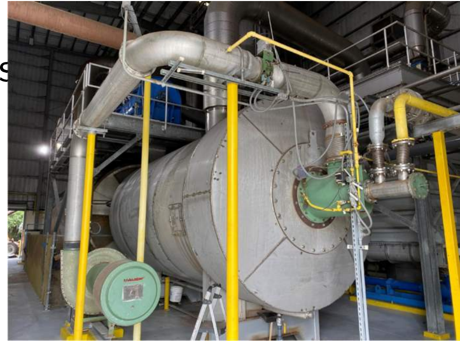
Manatee County Thermal Drum Dryer
