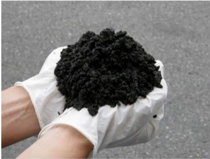
dewatered biosolids at 22% ds
