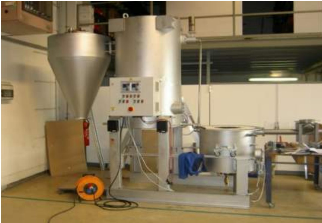
Type P-1: Throughput 45 lbs/hr at 70% ds
