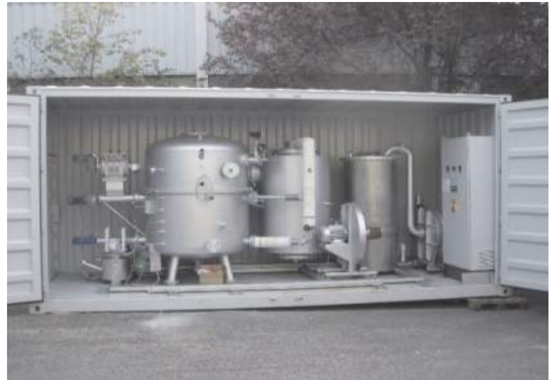
Type P-2: Throughput 220 lbs/hr at 70% ds
