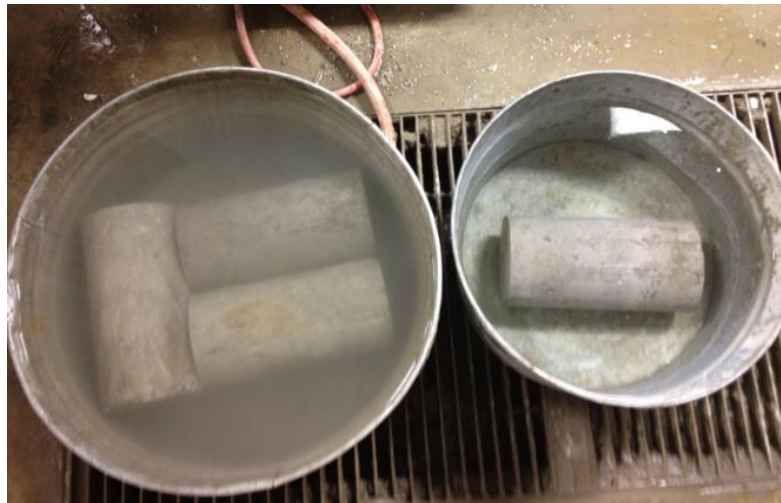
Concrete Coupons Curing
